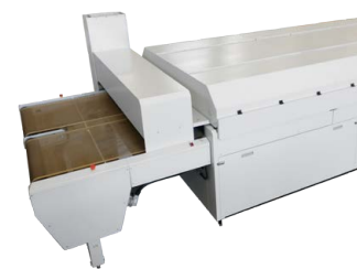
Exhaust fumes and outlet cooling hood
